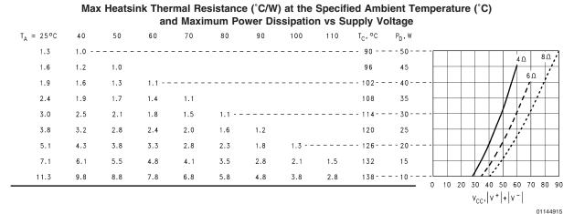
Note: The maximum heat sink thermal resistance values,  $Ø_{SA}$ , in the table above were calculated using a  $Ø_{CS} = 0.2^{\circ}C/W$  due to thermal compound.
