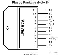
Top View Order Number LM3875T or LM3875TF See NS Package Number TA11B for Staggered Lead Non-Isolated Package or TF11B for Staggered Lead Isolated Package
